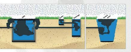
The Quick Oil System (QOS) stores the residual (oil and petrol) from the OWS separately in the reservoir.
